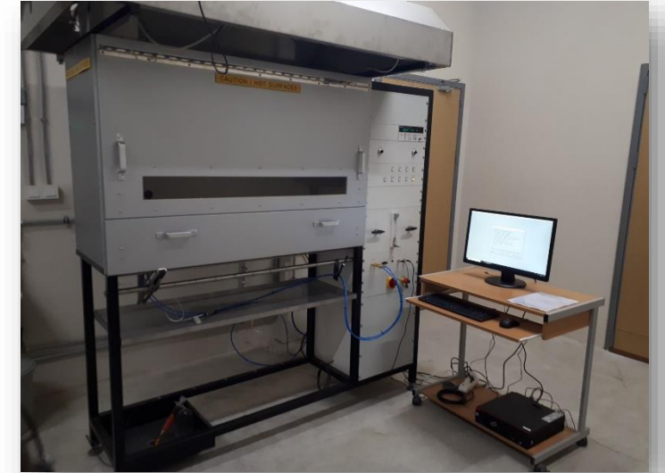
Flooring Radiant Panel ( EN ISO 9239-1 )
